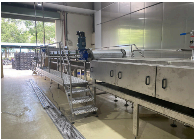
Fruit and vegetable blancher at a fruit juice plant in Vietnam, during installation. Kim Nguyen archive photo.
