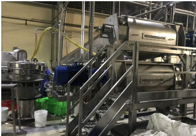
Fruit juice processing line: extractor, vibrating screen and conveyors, made in Italy.
