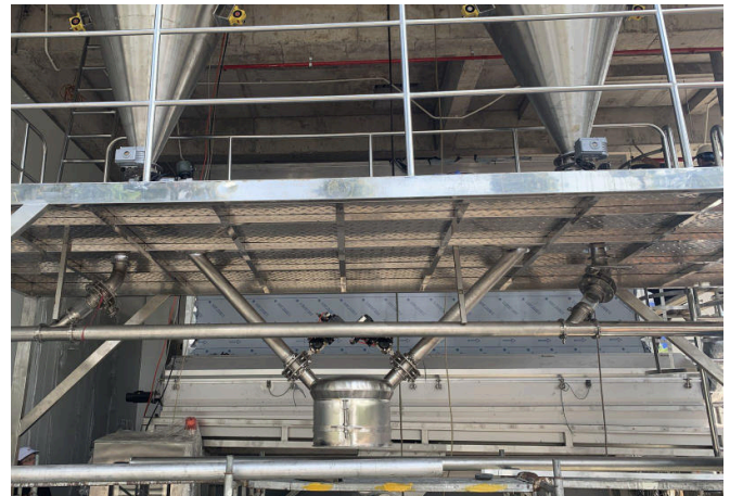
Upper level of the dryer with feed hoppers, made in the Netherlands.
