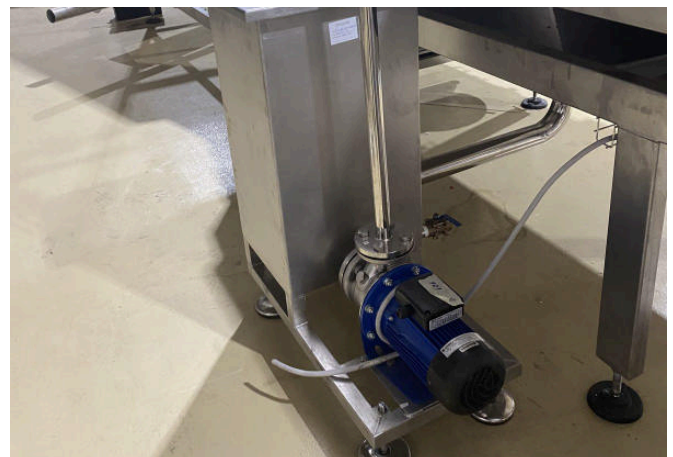
Stainless steel pump and hopper unit in the filling area. Kim Nguyen archive photo.
