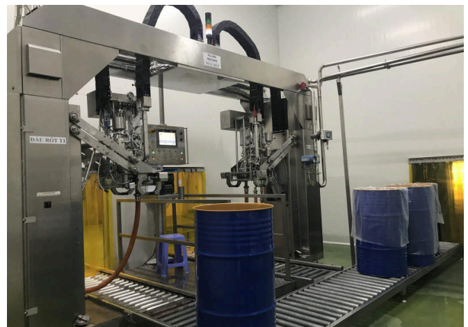
Aseptic drum filling station for export fruit juice concentrate. Kim Nguyen archive photo.
